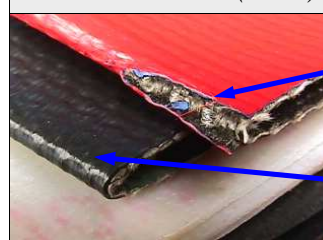
Cold Bend Test @ -90°F (-67.8°C)
