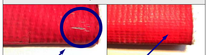
Hot Bend Test @ Temperatures Above 600°F (316.5°C)
