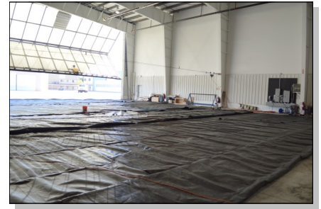
Fabrication of a large scale TCI CrossFilm™ secondary containment liner.
