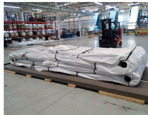
FIGURE 2 Shop fabricated PTFE liner accordion folded and ready for shipment and rapid deployment at site.
