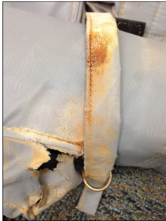
CHEMICALLY ATTACKED JACKETS PRODUCED USING PTFE COATED FIBERGLASS
