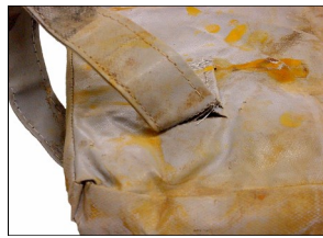
CHEMICALLY ATTACKED JACKETS PRODUCED USING PTFE COATED FIBERGLASS
