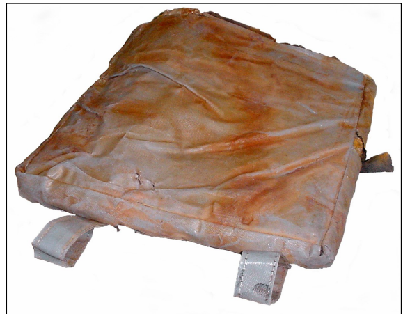
CHEMICALLY ATTACKED JACKETS PRODUCED USING PTFE COATED FIBERGLASS
